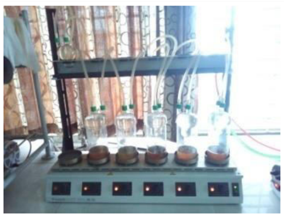
Fig. 4: Acid and Alkali digestion of feed sample.
