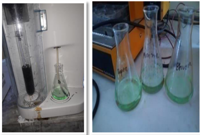
Fig. 5: Distillation process to detect crude protein.
